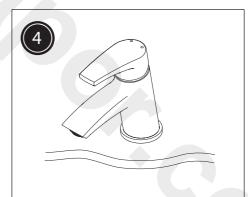
Connect the flexi tails to the hot and cold water supplies. Turn on the mains water supply letting the water flow for a few minutes to flush through the system. Check all joints and connections for any leaks.
